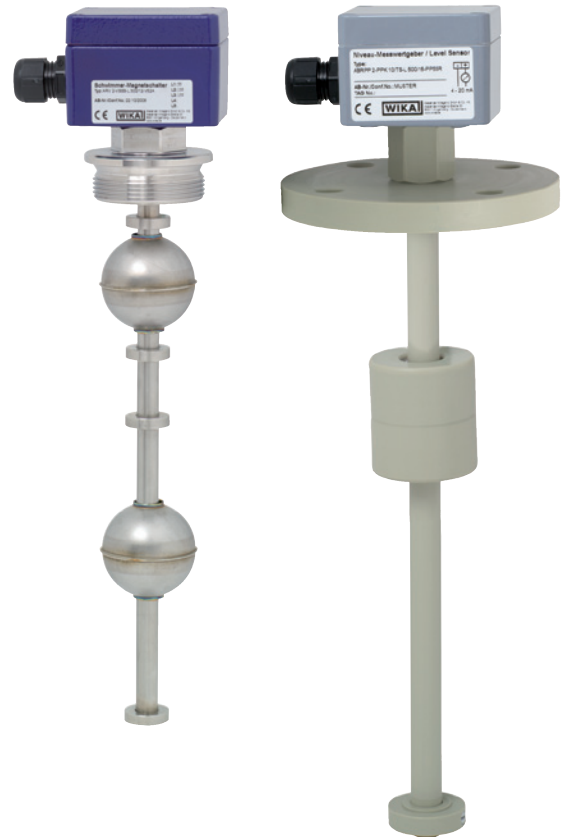
Float Switches with Permanent Magnet, for vertical installation, Model RSM Fig. left: Stainless steel version, mounting thread Fig. right: Plastic version, flange connection
